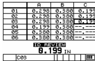
Step 2: Use [↑, ↓, ←, →] to move to a new grid or ID# location. For incremental or sequential files, only the [↑, ↓] keys can be used.
