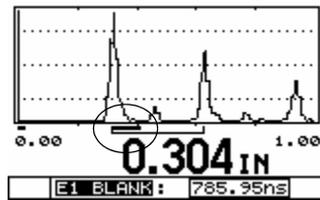
**E1 (Echo1) Blank Set Properly; Gage Making Proper Detection Between Successive Backwall Echoes**
