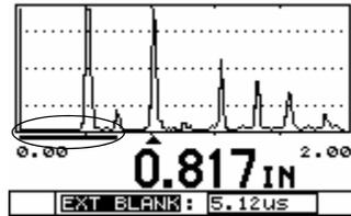
**Gage Measuring First Echo Over the 20% Gradicule After the End of the Extended Blank**
