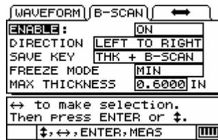
Once the B-scan function has been enabled, the B-scan starts drawing the cross-sectional thickness when the transducer make contact with the material and the first thickness reading is displayed. The B-scan will continue to draw while displaying the live thickness at the transducer location until one of the following events occurs:
