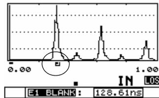
**Echo Blank Set Too Small; Gage Reading Trailing Edge of First Backwall Echo**
