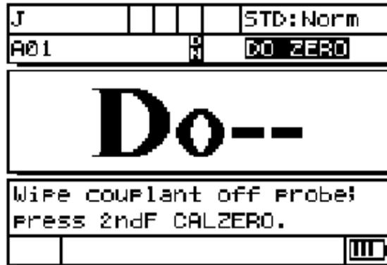
**Figure 2-1: Transducer ZERO Compensation**
