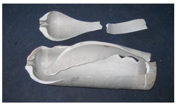
This is the latest in a number of incidents involving the filling of aluminium SCUBA cylinders manufactured from 6351 alloy. The 6351 alloy was used in:
